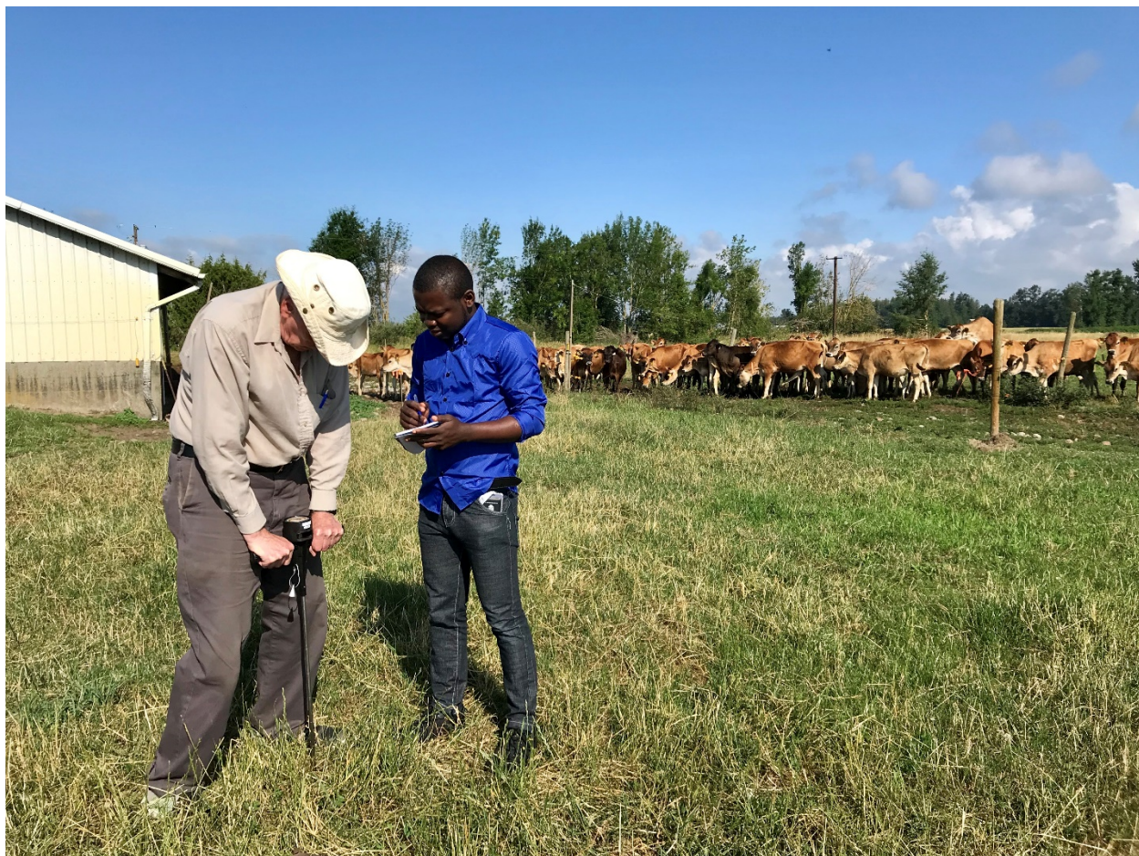
Figure 2 Student Bosun Ayetan and Prof Les Lavkulich taking soil compaction measurements with a penetrometer (June 2019)
